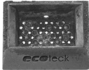
Basket needing cleaning with the holes blocked by ashes
